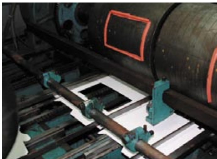
A die is used to cut a space in the carton for a film window that displays the product.
